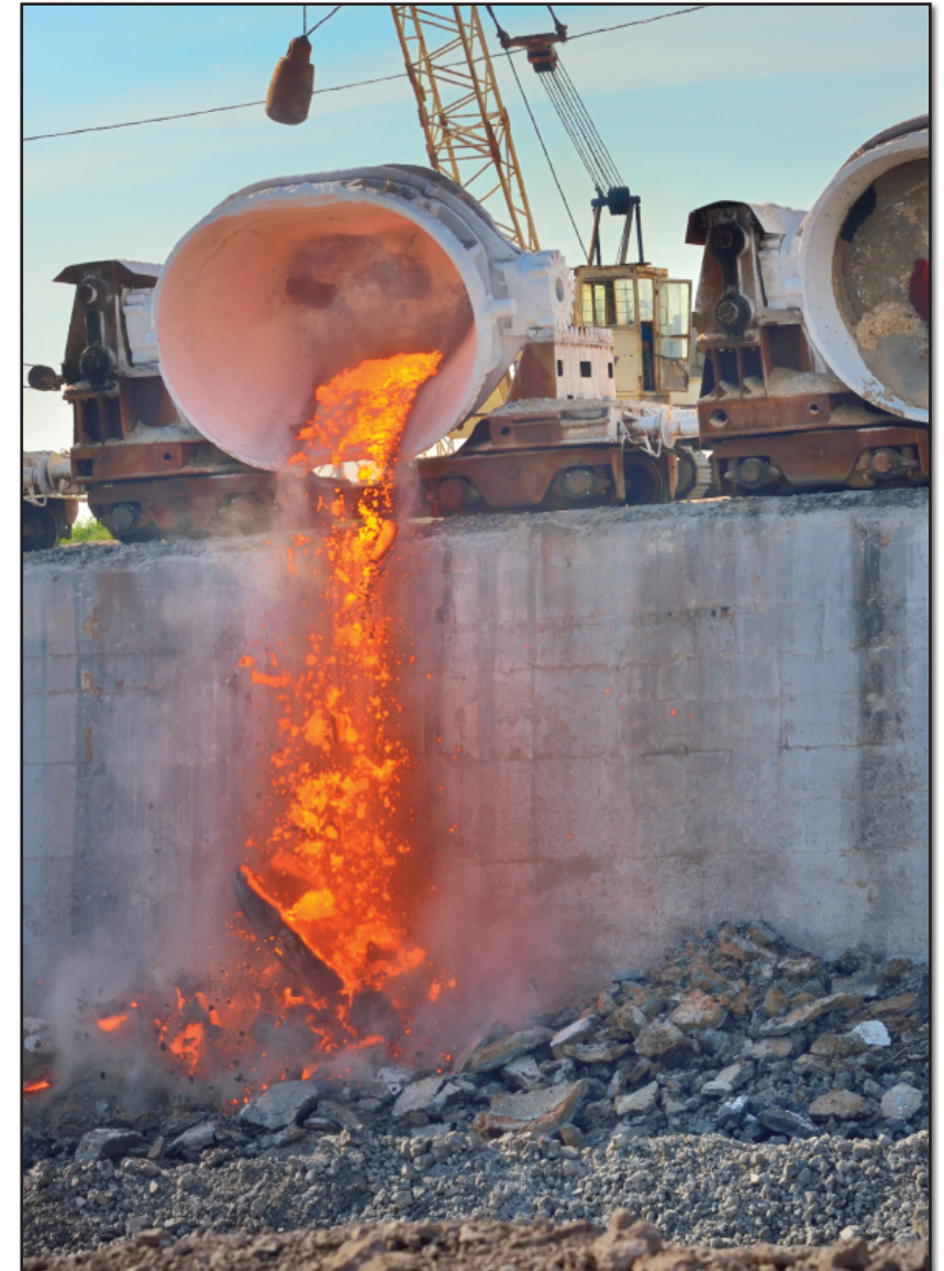
Slag is poured into a pit to cool.
