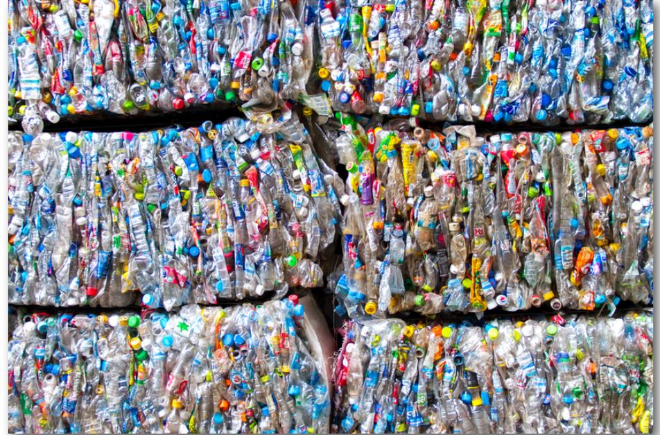
The blocks are then shredded. The tiny pieces of old plastic are washed and melted to form a resin once again. The resin is cut into new pellets ready to be sold to manufacturers.
