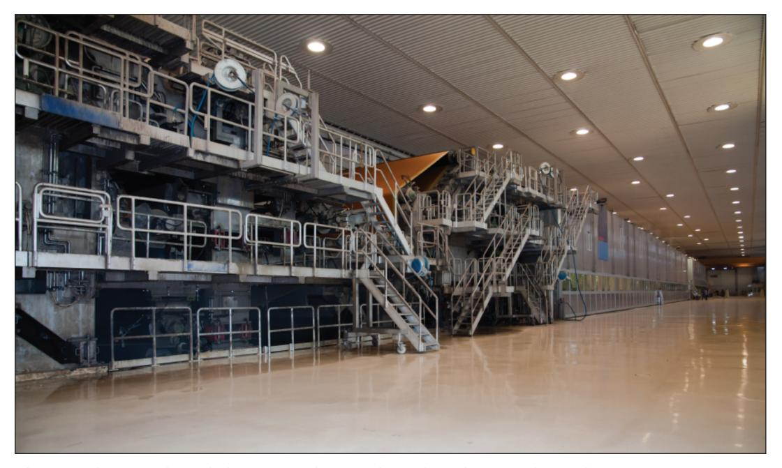
The wet pulp is sent through the paper making machine. The pulp enters the machine as a continuous stream. First, it is poured onto a on a wire mesh so that excess water can drain through. Then the paper moves through a series of pressing rollers and driers until it reaches the end of the machine.
