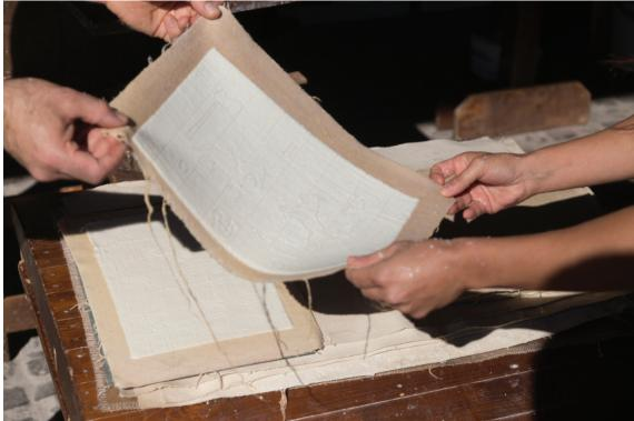
The top frame is removed and the meshed frame, containing the wet paper pulp, is flipped onto a piece of cloth. The wet paper sticks to the cloth.
