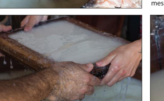
• The paper making frame consists of a set of two frames. The bottom one contains a fine wire mesh, the top one forms the border for the paper.
